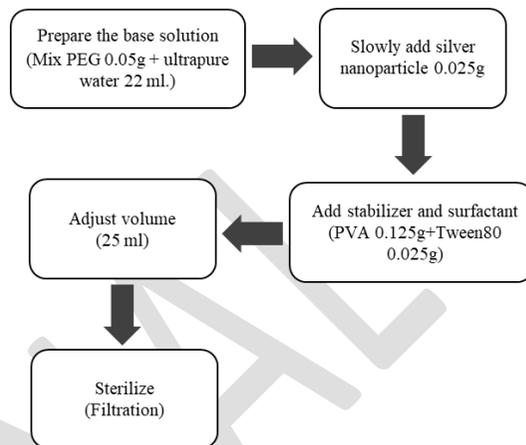
**Fig. 1.** Preparation of silver nanoparticle microemulsion involving a five-step procedure.
